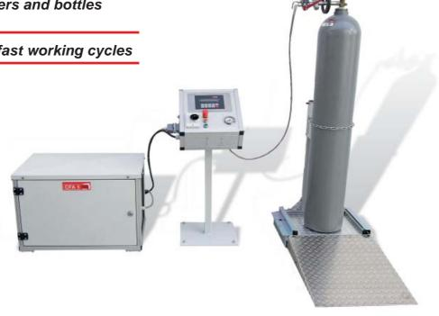
Fig. 1: The CFA 5 Carbon Dioxide Filling Unit is designed for the precise filling of CO<sub>2</sub> from the liquid phase. It is used to fill CO, bottles from 2 to 50 kg with cryogenic carbon dioxide from low-pressure tanks (15 to 20 bar).
