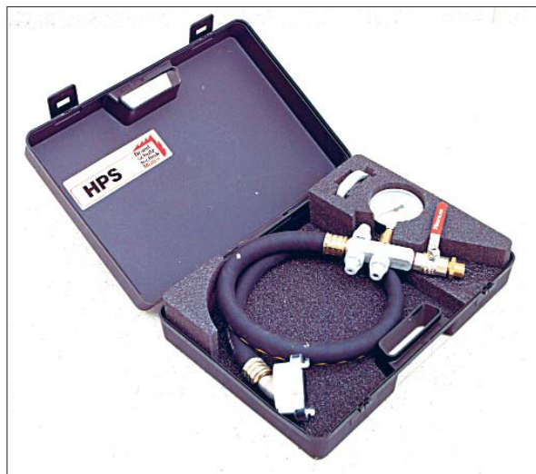
Fig. 7: With the HPS Hydrant Testing Set both the pressure at rest and the flow pressure of the extinguishing water can be measured on rising mains.
